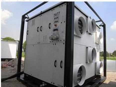
The Climate Control Air Handling Unit.
